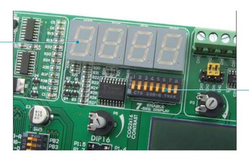
DIP switch SW10 turns the seven-segment display digits on
